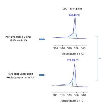
Parts produced using 3M<sup>TM</sup> and Replacement fine powders have similar melt peaks. This result indicates that the 3M<sup>TM</sup> resin YY and Replacement resin AA respond similarly when exposed to the same heating conditions. The conclusion from this data is that replacement resin has not been thermally degraded or unexpectedly altered during the manufacture of PTFE Dual-Shrink<sup>TM</sup>.
