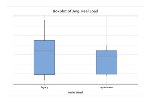
Testing demonstrated that replacement resins uphold existing contact angle requirements on all etched extrusions. The peel testing on Part 2 shows similar adhesion between the PTFE liner and the poly(ether-block-amide) outer jacket.
