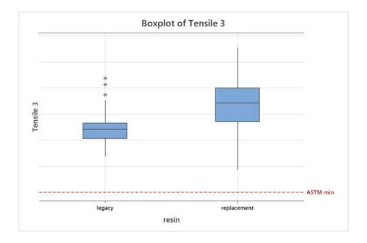
Part 2 (ID 0.097"/Wall 0.0015") has similar tensile properties vs. the same part when run with the legacy resin. All burst values maxed out the text fixture at 99.9 PSI.
