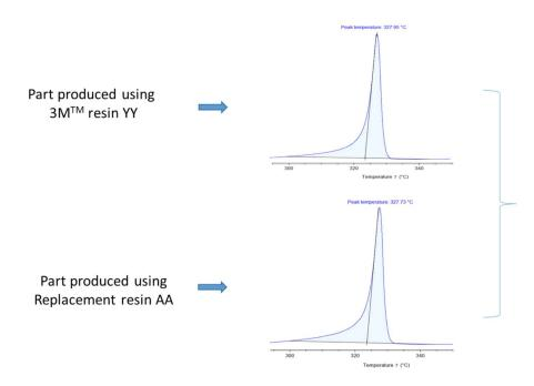
Parts produced using 3M<sup>TM</sup> and Replacement fine powders have similar melt peaks. This result indicates that the 3M resin YY and Replacement resin AA respond similarly when exposed to the same heating conditions. The conclusion from this data is that replacement resin has not been thermally degraded or unexpectedly altered during the manufacture of an extruded PTFE liner.
