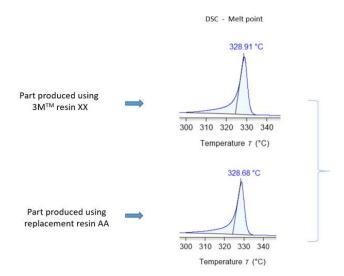
Parts produced using 3M<sup>™</sup> and Replacement fine powders have similar melt peaks. This result indicates that the 3M<sup>™</sup> resin YY and Replacement resin AA respond similarly when exposed to the same heating conditions. The conclusion from this data is that replacement resin has not been thermally degraded or unexpectedly altered during the manufacture of PTFE Heat Shrink.
