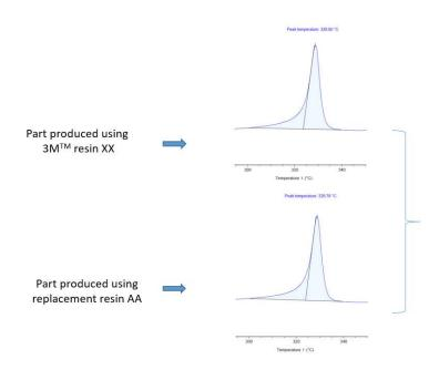
Parts produced using 3M™ and Replacement fine powders have similar melt peaks. This result indicates that the 3M resin XX and replacement resin AA respond similarly when exposed to the same heating conditions. The conclusion from this data is that replacement resin has not been thermally degraded or unexpectedly altered during the manufacture of PTFE tubing.
