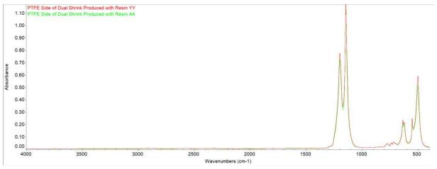
The peaks present in the replacement resin overlay with the peaks from the other PTFE resins and align with the functional group vibrations for PTFE. There are no additional peaks present, which would indicate differences in material composition or contamination.
