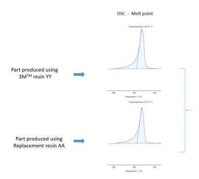
Parts produced using 3M<sup>™</sup> and replacement fine powders have similar melt peaks. This result indicates that the 3M resin YY and replacement resin AA respond similarly when exposed to the same heating conditions. The conclusion from this data is that replacement resin has not been thermally degraded or unexpectedly altered during the manufacture of an extruded, pigmented, flared PTFE product.
