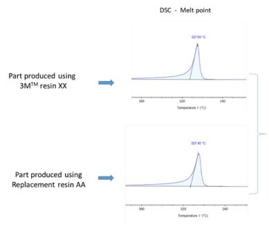
Parts produced using 3M<sup>TM</sup> and Replacement fine powders have similar melt peaks. This result indicates that the 3M resin XX and Replacement resin AA respond similarly when exposed to the same heating conditions. The conclusion from this data is that replacement resin has not been thermally degraded or unexpectedly altered during the manufacture of an extruded PTFE liner.
