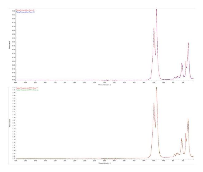
The peaks present in the replacement resin overlay with the peaks from the other PTFE resins and align with the functional group vibrations for PTFE. There are no additional peaks present, which would indicate differences in material composition or contamination.
