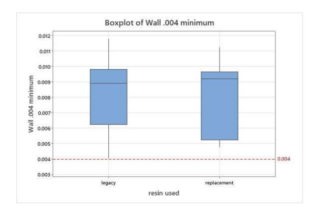
For this multi-lumen part, the ODs are extruded towards the upper specification limit and IDs towards the lower specification limit to maximize wall thickness at customer request. IDs are accepted on an attribute pass/fail basis.
